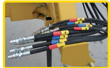
8 pcs. hoses connected properly within 2 min.
